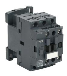
Schneider Electric Easy TeSys series IEC contactor, 12A, (3) N.O. power poles, (1) N.O. auxiliary contacts, 120 VAC (50/60Hz) coil voltage.
