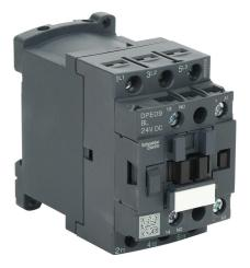
Schneider Electric Easy TeSys series IEC contactor, 9A, (3) N.O. power poles, (1) N.O. auxiliary contacts, 24 VDC coil voltage.
