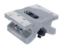
PBC DPB series double roller pillow block, cam follower bearing, 3.37in overall length, steel, 1-1/4in inside diameter, aluminum housing, adjustable running clearance. For use with 1-1/4in diameter PBC shafts.
