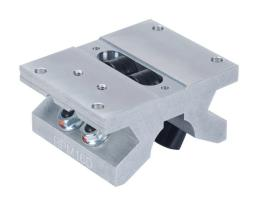
PBC DPB series double roller pillow block, cam follower bearing, 2.62in overall length, steel, 1in inside diameter, aluminum housing, adjustable running clearance. For use with 1in diameter PBC shafts.
