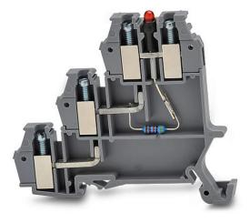
DINnector screw triple-level sensor terminal block, power indicator, accepts wire size 26-14 AWG, gray, 10A, PNP LED indicator(s), 35mm DIN rail mount, 10kA SCCR. Package of 25.
