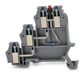
DINnector screw triple-level sensor terminal block, power indicator, accepts wire size 26-14 AWG, gray, 10A, PNP LED indicator(s), 35mm DIN rail mount, 10kA SCCR. Package of 25.
