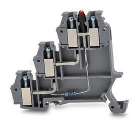
DINnector screw triple-level sensor terminal block, power indicator, accepts wire size 26-14 AWG, gray, 10A, NPN LED indicator(s), 35mm DIN rail mount, 10kA SCCR. Package of 25.
