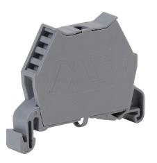
DINnector screw thermocouple terminal block, accepts wire size 30-20 AWG, gray, 35mm DIN rail mount, 10kA SCCR. Package of 10.
