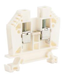
DINnector screw single-level feedthrough terminal block, accepts wire size 22-8 AWG, white, 50A, 35mm DIN rail mount, 100kA SCCR. Package of 50.
