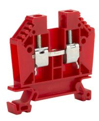
DINnector screw single-level feedthrough terminal block, accepts wire size 22-8 AWG, red, 50A, 35mm DIN rail mount, 100kA SCCR. Package of 50.
