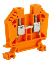
DINnector screw single-level feedthrough terminal block, accepts wire size 22-8 AWG, orange, 50A, 35mm DIN rail mount, 100kA SCCR. Package of 50.
