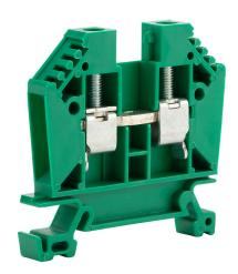
DINnector screw single-level feedthrough terminal block, accepts wire size 22-8 AWG, green, 50A, 35mm DIN rail mount, 100kA SCCR. Package of 50.
