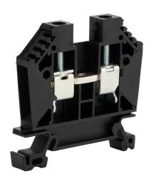
DINnector screw single-level feedthrough terminal block, accepts wire size 22-8 AWG, black, 50A, 35mm DIN rail mount, 100kA SCCR. Package of 50.
