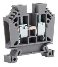
DINnector screw single-level feedthrough terminal block, accepts wire size 18-6 AWG, gray, 65A, 35mm DIN rail mount, 100kA SCCR. Package of 50.
