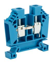
DINnector screw single-level feedthrough terminal block, accepts wire size 18-6 AWG, blue, 65A, 35mm DIN rail mount, 100kA SCCR. Package of 50.
