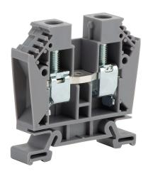
DINnector screw single-level feedthrough terminal block, accepts wire size 14-4 AWG, gray, 85A, 35mm DIN rail mount, 100kA SCCR. Package of 25.
