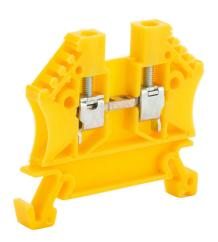
DINnector screw single-level feedthrough terminal block, accepts wire size 24-12 AWG, yellow, 20A, 35mm DIN rail mount, 100kA SCCR. Package of 100. For use with jumpers DN-24J2Y, DN-2J2Y and DN-3J2Y.
