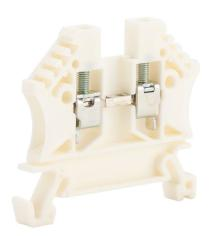
DINnector screw single-level feedthrough terminal block, accepts wire size 24-12 AWG, white, 20A, 35mm DIN rail mount, 100kA SCCR. Package of 100. For use with jumpers DN-24J2Y, DN-2J2Y and DN-3J2Y.
