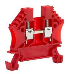
DINnector screw single-level feedthrough terminal block, accepts wire size 24-12 AWG, red, 20A, 35mm DIN rail mount, 100kA SCCR. Package of 100. For use with jumpers DN-24J2Y, DN-2J2Y and DN-3J2Y.
