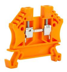
DINnector screw single-level feedthrough terminal block, accepts wire size 24-12 AWG, orange, 20A, 35mm DIN rail mount, 100kA SCCR. Package of 100. For use with jumpers DN-24J2Y, DN-2J2Y and DN-3J2Y.
