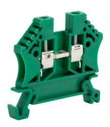
DINnector screw single-level feedthrough terminal block, accepts wire size 24-12 AWG, green, 20A, 35mm DIN rail mount, 100kA SCCR. Package of 100. For use with jumpers DN-24J2Y, DN-2J2Y and DN-3J2Y.
