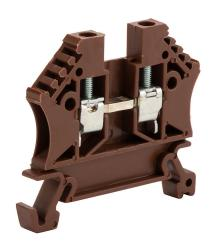
DINnector screw single-level feedthrough terminal block, accepts wire size 24-12 AWG, brown, 20A, 35mm DIN rail mount, 100kA SCCR. Package of 100. For use with jumpers DN-24J2Y, DN-2J2Y and DN-3J2Y.
