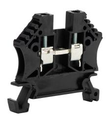
DINnector screw single-level feedthrough terminal block, accepts wire size 24-12 AWG, black, 20A, 35mm DIN rail mount, 100kA SCCR. Package of 100. For use with jumpers DN-24J2Y, DN-2J2Y and DN-3J2Y.
