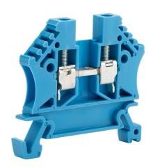
DINnector screw single-level feedthrough terminal block, accepts wire size 24-12 AWG, blue, 20A, 35mm DIN rail mount, 100kA SCCR. Package of 100. For use with jumpers DN-24J2Y, DN-2J2Y and DN-3J2Y.
