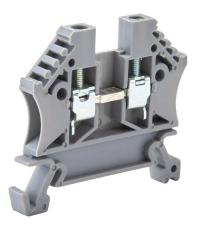
DINnector screw single-level feedthrough terminal block, accepts wire size 24-12 AWG, gray, 20A, 35mm DIN rail mount, 100kA SCCR. Package of 100. For use with jumpers DN-24J2Y, DN-2J2Y and DN-3J2Y.
