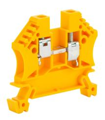
DINnector screw single-level feedthrough terminal block, accepts wire size 24-10 AWG, yellow, 30A, 35mm DIN rail mount, 100kA SCCR. Package of 100. For use with jumpers DN-24J4Y, DN-2J4Y and DN-3J4Y.
