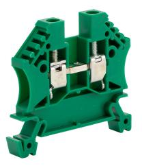
DINnector screw single-level feedthrough terminal block, accepts wire size 24-10 AWG, green, 30A, 35mm DIN rail mount, 100kA SCCR. Package of 100. For use with jumpers DN-24J4Y, DN-2J4Y and DN-3J4Y.
