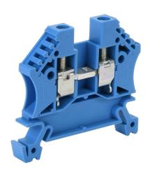
DINnector screw single-level feedthrough terminal block, accepts wire size 24-10 AWG, blue, 30A, 35mm DIN rail mount, 100kA SCCR. Package of 100. For use with jumpers DN-24J4Y, DN-2J4Y and DN-3J4Y.
