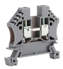
DINnector screw single-level feedthrough terminal block, accepts wire size 24-10 AWG, gray, 30A, 35mm DIN rail mount, 100kA SCCR. Package of 100. For use with jumpers DN-24J4Y, DN-2J4Y and DN-3J4Y.
