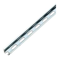
DINnector DIN rail, slotted, 15mm width, 5.5mm height, 1m length, plated steel. Package of 2.
