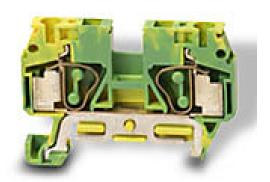
DINnector screwless grounding terminal block, accepts wire size 24-10 AWG, green and yellow, 35mm DIN rail mount, 10kA SCCR. Package of 10. Use to mechanically and electrically connect wires to 35mm DIN rail through the clamping foot.
