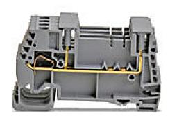
DINnector screwless plug-in single-level feedthrough terminal block, accepts wire size 24-12 AWG, gray, 12A, 35mm DIN rail mount, 10kA SCCR. Package of 32.
