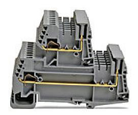
DINnector screwless plug-in double-level feedthrough terminal block, accepts wire size 24-12 AWG, gray, 12A, 35mm DIN rail mount, 10kA SCCR. Package of 32.
