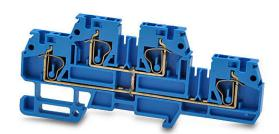
DINnector screwless double-level feedthrough terminal block, connected between levels, accepts wire size 24-12 AWG, blue, 20A, 35mm DIN rail mount, 10kA SCCR. Package of 10. For use with jumpers DN-24J2Y, DN-2J2Y or DN-3J2Y.
