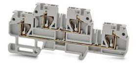
DINnector screwless double-level feedthrough terminal block, connected between levels, accepts wire size 24-12 AWG, gray, 20A, 35mm DIN rail mount, 10kA SCCR. Package of 10. For use with jumpers DN-24J2Y, DN-2J2Y or DN-3J2Y.
