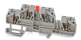
DINnector screwless double-level feedthrough terminal block, connected between levels and power indicator, accepts wire size 24-12 AWG, gray, 20A, 12-24 VAC/VDC LED indicator(s), 35mm DIN rail mount, 10kA SCCR. Package of 10.
