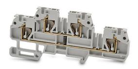
DINnector screwless double-level feedthrough terminal block, connected between levels and diode, accepts wire size 24-12 AWG, gray, 20A, 35mm DIN rail mount, 10kA SCCR. Package of 10. For use with jumpers DN-24J2Y, DN-2J2Y or DN-3J2Y.
