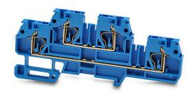
DINnector screwless double-level feedthrough terminal block, accepts wire size 24-12 AWG, blue, 20A, 35mm DIN rail mount, 10kA SCCR. Package of 25. For use with jumpers DN-24J2Y, DN-2J2Y or DN-3J2Y.
