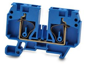
DINnector screwless single-level feedthrough terminal block, accepts wire size 22-8 AWG, blue, 45A, 35mm DIN rail mount, 10kA SCCR. Package of 50. For use with jumpers DN-12J6Y, DN-2J6Y or DN-3J6Y.
