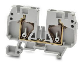
DINnector screwless single-level feedthrough terminal block, accepts wire size 22-8 AWG, gray, 45A, 35mm DIN rail mount, 10kA SCCR. Package of 50. For use with jumpers DN-12J6Y, DN-2J6Y or DN-3J6Y.
