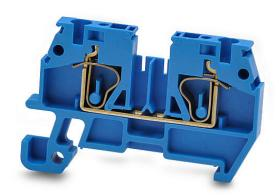
DINnector screwless single-level feedthrough terminal block, accepts wire size 24-12 AWG, blue, 20A, 35mm DIN rail mount, 10kA SCCR. Package of 50. For use with jumpers DN-24J2Y, DN-2J2Y or DN-3J2Y.
