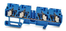
DINnector screwless common point single-level feedthrough terminal block, two-connection to two-connection, accepts wire size 24-12 AWG, blue, 20A, 35mm DIN rail mount, 10kA SCCR. Package of 25. For use with jumpers DN-24J2Y, DN-2J2Y or DN-3J2Y.
