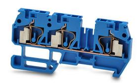
DINnector screwless common point single-level feedthrough terminal block, one-connection to two-connection, accepts wire size 24-12 AWG, blue, 20A, 35mm DIN rail mount, 10kA SCCR. Package of 25. For use with jumpers DN-24J2Y, DN-2J2Y or DN-3J2Y.
