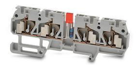
DINnector screwless common point single-level feedthrough terminal block, two-connection to two-connection and power indicator, accepts wire size 24-12 AWG, gray, 20A, 12-24 VAC/VDC LED indicator(s), 35mm DIN rail mount, 10kA SCCR. Package of 10.
