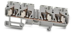
DINnector screwless common point single-level feedthrough terminal block, two-connection to two-connection, accepts wire size 24-12 AWG, gray, 20A, 35mm DIN rail mount, 10kA SCCR. Package of 25. For use with jumpers DN-24J2Y, DN-2J2Y or DN-3J2Y.
