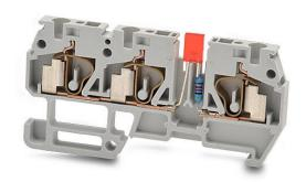
DINnector screwless common point single-level feedthrough terminal block, power indicator, accepts wire size 24-12 AWG, gray, 20A, 12-24 VAC/VDC LED indicator(s), 35mm DIN rail mount, 10kA SCCR. Package of 10.
