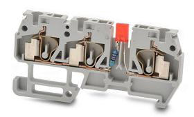
DINnector screwless common point single-level feedthrough terminal block, one-connection to two-connection and power indicator, accepts wire size 24-12 AWG, gray, 20A, 12-24 VAC/VDC LED indicator(s), 35mm DIN rail mount, 10kA SCCR. Package of 10.
