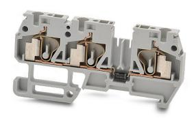
DINnector screwless common point single-level feedthrough terminal block, diode, accepts wire size 24-12 AWG, gray, 20A, 35mm DIN rail mount, 10kA SCCR. Package of 10. For use with jumpers DN-24J2Y, DN-2J2Y or DN-3J2Y.
