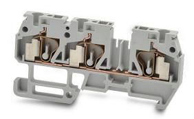
DINnector screwless common point single-level feedthrough terminal block, one-connection to two-connection, accepts wire size 24-12 AWG, gray, 20A, 35mm DIN rail mount, 10kA SCCR. Package of 25. For use with jumpers DN-24J2Y, DN-2J2Y or DN-3J2Y.
