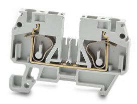
DINnector screwless single-level feedthrough terminal block, accepts wire size 24-10 AWG, gray, 30A, 35mm DIN rail mount, 10kA SCCR. Package of 50. For use with jumpers DN-24J4Y, DN-2J4Y and DN-3J4Y.
