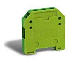
DIN*nector* screw mini grounding terminal block, accepts wire size 24-10 AWG, green and yellow, 15mm DIN rail mount, 10kA SCCR. Package of 20. Use to mechanically and electrically connect wires to 15mm DIN rail through the screw-down clamping foot.
